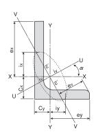
Geometrical of inertia l=ai2 Radius of gyration of area  $i=\sqrt{1/a}$ Modulus of section Z=1/e
